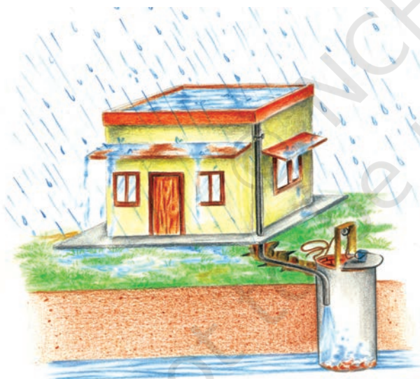
(b) Recharge through Abandoned Dugwell
