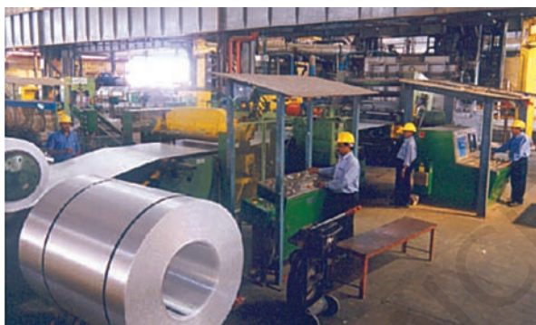
Fig. 6.3: Strip coating mill at smelter of NALCO
