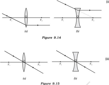
(ii) A ray of light passing through a principal focus, after refraction from a convex lens, will emerge parallel to the principal axis. This is shown in Fig. 9.14 (a). A ray of light appearing to meet at the principal focus of a concave lens, after refraction, will emerge parallel to the principal axis. This is shown in Fig.9.14 (b).
