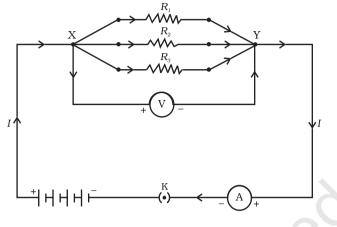
Figure 11.7 Resistors in parallel
