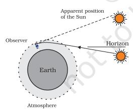
Figure 10.10 Atmospheric refraction effects at sunrise and sunset Why don't the planets twinkle? The planets are much closer to the earth, and are thus seen as extended sources. If we consider a planet as a collection of a large number of point-sized sources of light, the total variation in the amount of light entering our eye from all the individual point-sized sources will average out to zero, thereby nullifying the twinkling effect.
