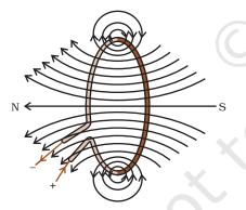
**Figure 12.8** Magnetic field lines of the field produced by a current-carrying circular loop
