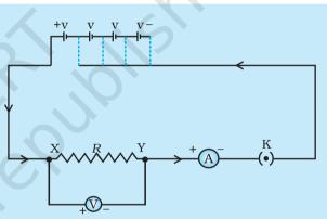
Figure 11.2 Electric circuit for studying Ohm's law
