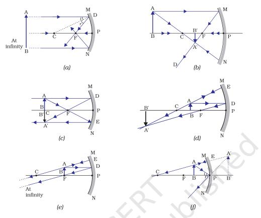
Figure 9.7 Ray diagrams for the image formation by a concave mirror
