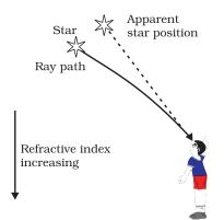
Figure 10.9 Apparent star position due to atmospheric refraction
