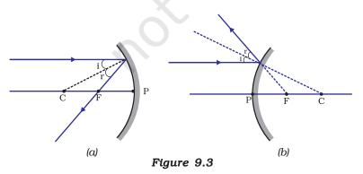
(i) A ray parallel to the principal axis, after reflection, will pass through the principal focus in case of a concave mirror or appear to diverge from the principal focus in case of a convex mirror. This is illustrated in Fig.9.3 (a) and (b).
