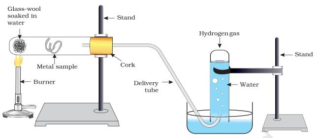
Figure 3.3 Action of steam on a metal
