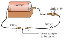
Figure 3.2 Metals are good conductors of electricity.
