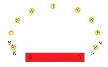
*Figure 12.3* Drawing a magnetic field line with the help of a compass needle
