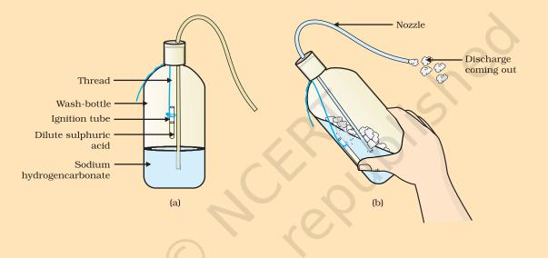
*Figure 2.10* (a) Ignition tube containing dilute sulphuric acid suspended in a wash-bottle containing sodium hydrogencarbonate, (b) Discharge coming out of the nozzle
