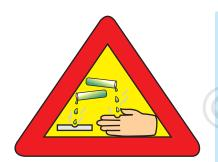
Figure 2.5 Warning sign displayed on containers containing concentrated acids and bases
