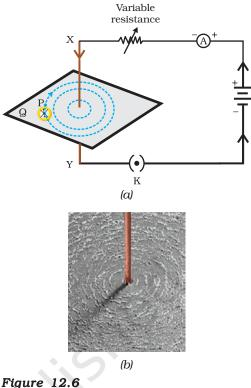
(a) A pattern of concentric circles indicating the field lines of a magnetic field around a straight conducting wire. The arrows in the circles show the direction of the field lines.
