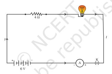
Figure 11.9 An electric lamp connected in series with a resistor of 4  $\Omega$  to a 6 V battery
