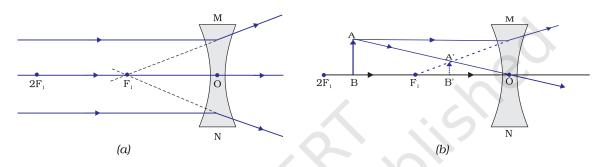
Figure 9.17 Nature, position and relative size of the image formed by a concave lens
