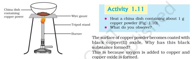
Figure 1.10 Oxidation of copper to copper oxide
