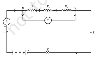
Figure 11.6 Resistors in series
