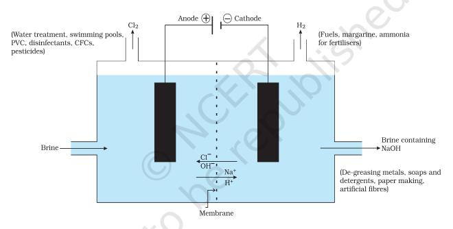
Figure 2.8 Important products from the chlor-alkali process
